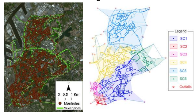
Figure 2: Detailed 1D-2D InfoWorks ICM model of the case study area (left) and hydraulic conceptual CMD model (right).
